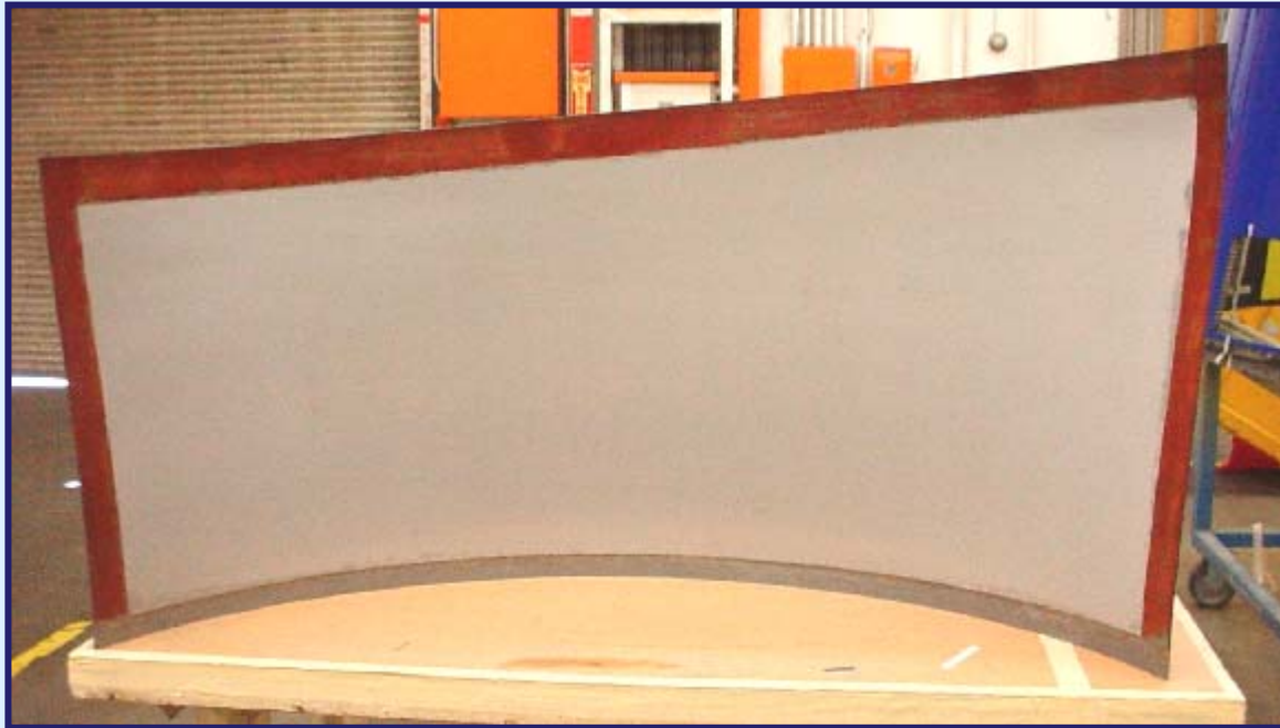
Inlet Cowl Inner Barrel Panel (composite construction)
